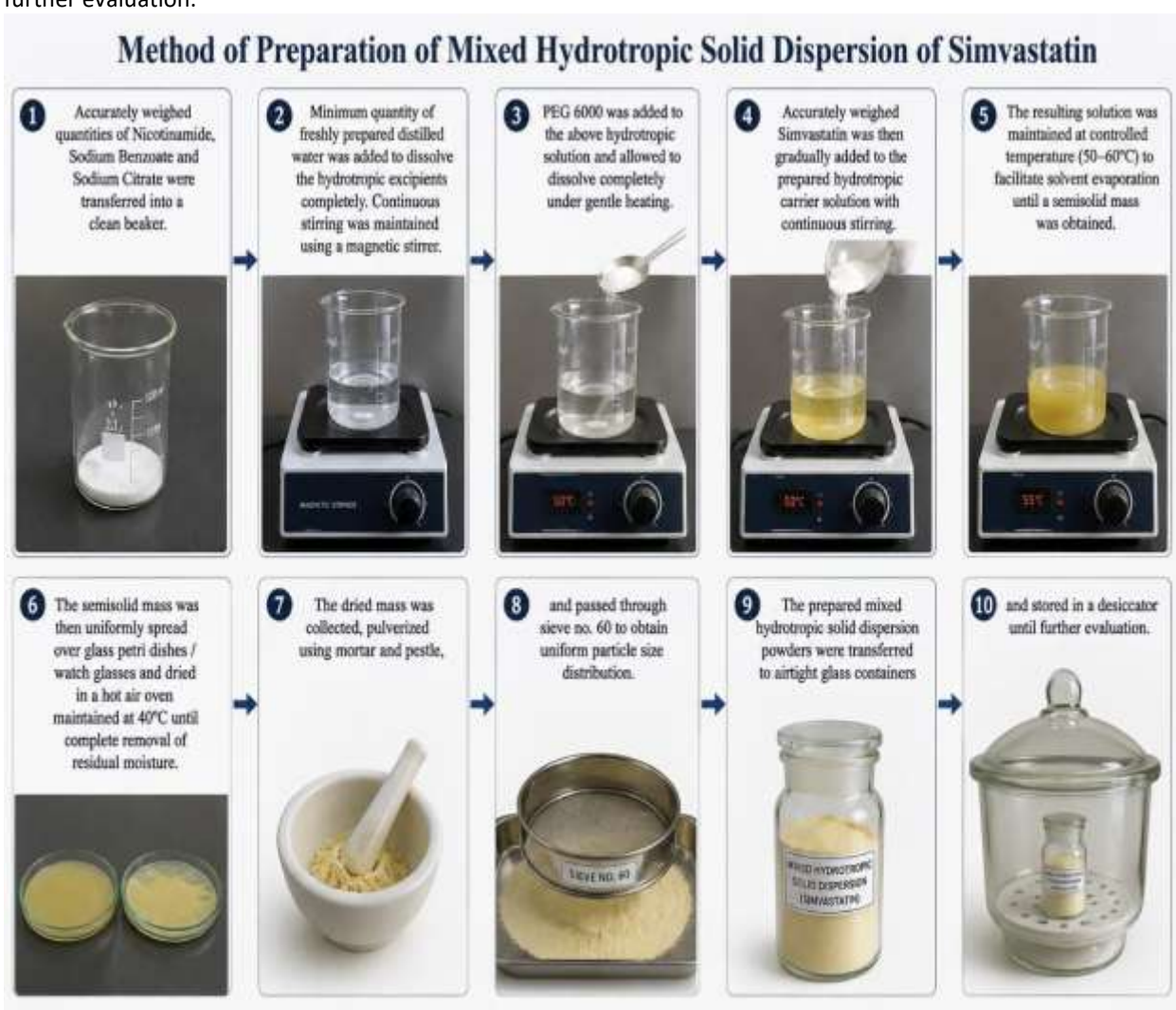
Figure 1: Schematic representation of the preparation method for Simvastatin mixed hydrotropic solid dispersion by solvent evaporation technique.
