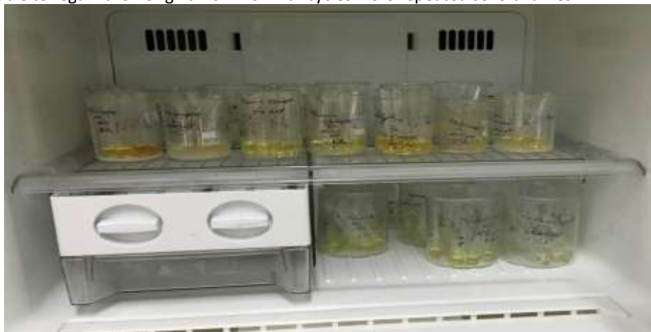
Fig. 1: Freeze thaw cycle application over formulations
