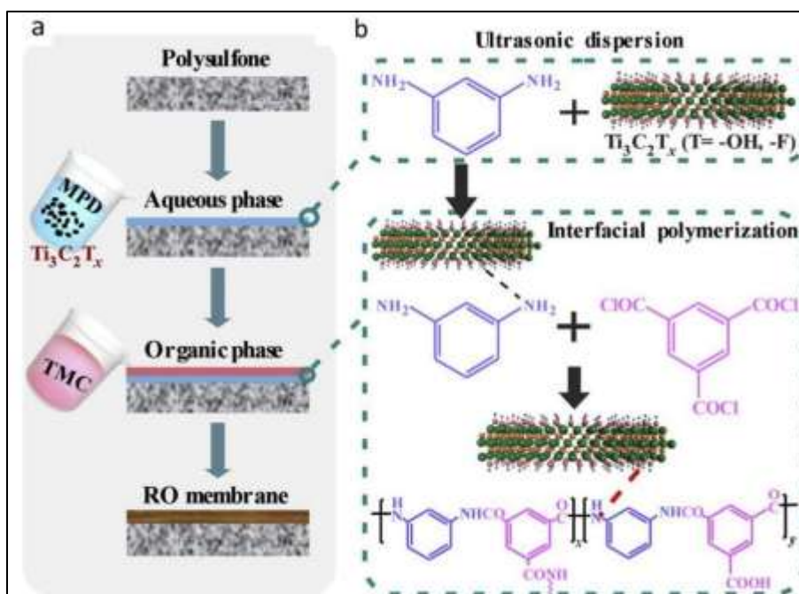
Fig. 8 (a) Schematic representation of the fabrication process for Ti_3C_2T_x -incorporated polyamide reverse osmosis (RO) membranes.
