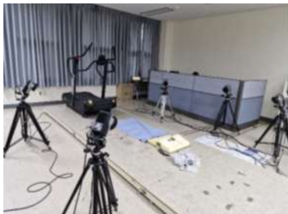
Figure 1. Five-camera Qualisys three-dimensional motion analysis system
