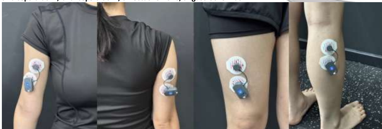
Figure 4. Location of electrodes a: biceps brachii, b: triceps brachii, c: rectus femoris, d: gastrocnemius
