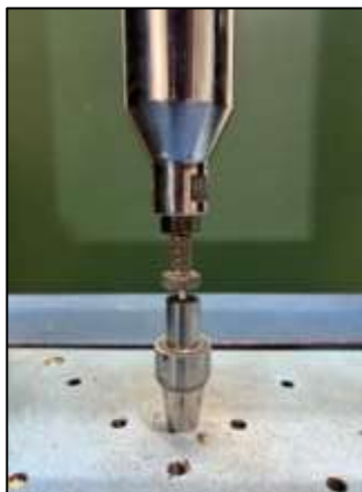
Fig. 3. Compression strength testing using UTM
