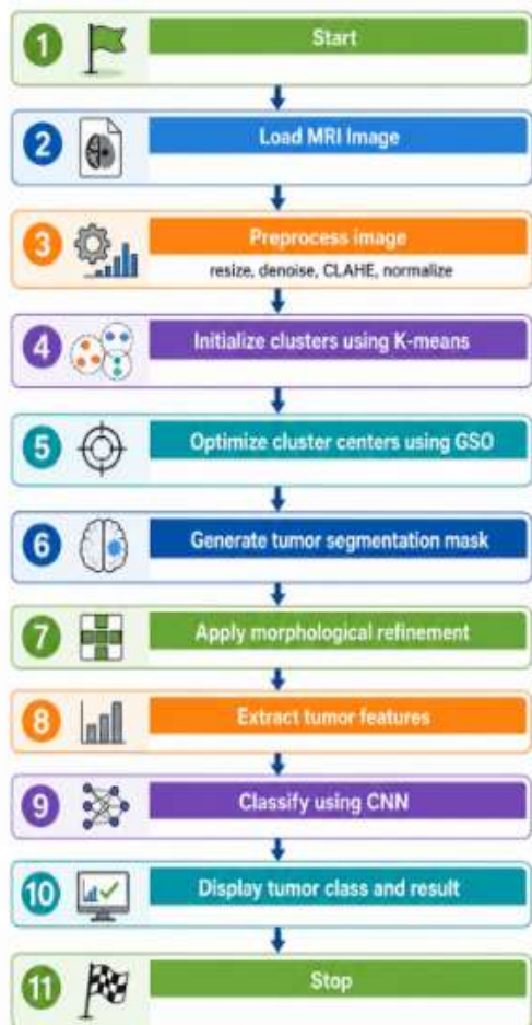
Fig. 2. Flowchart of the proposed CNN and KCGSO-based brain tumor detection method.
