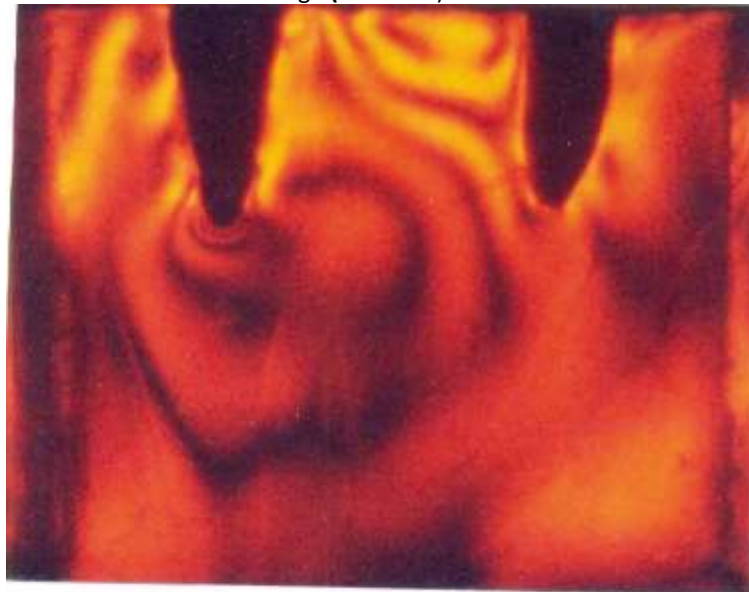
Stress Fringes for Bar-Clip Type of Overdenture at 50 lb.
