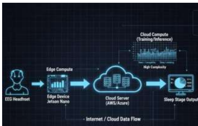
Fig. 10. Edge/cloud deployment concept for EEG-based sleep-stage classification.
