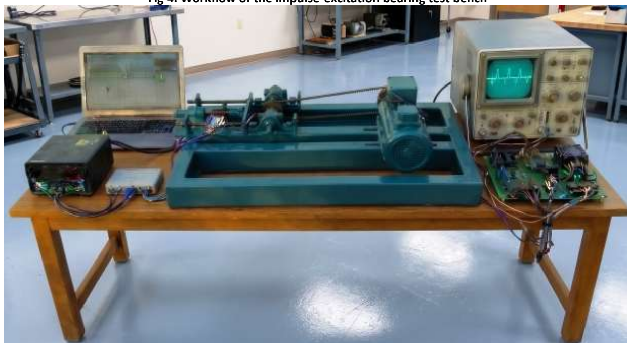
Fig 5. Experiment test bench: solenoid-driven, rubber-tipped plunger striking the inner race, ADXL335 accelerometer on the outer race, and the PSoC–LabVIEW acquisition system
