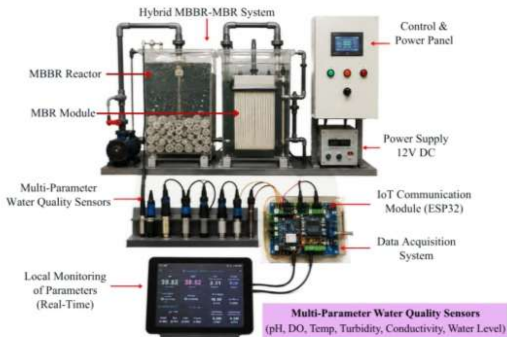
Figure 2. MBBR-MBR Technology in Wastewater Treatment
