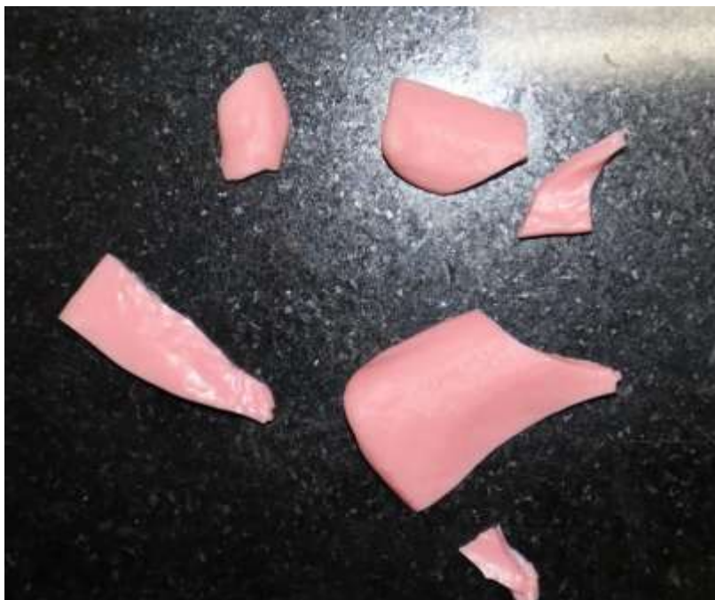
Fractured denture base
